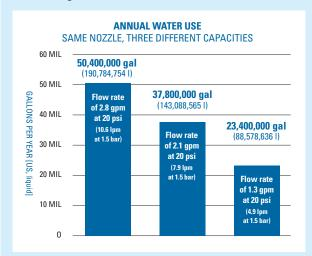
Based on 150 full cone spray nozzles spraying eight hours per day, five days per week, 50 weeks per year. 3/8" H FullJet® nozzle used for the comparison.
