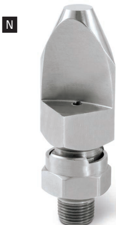
OLPA Spray Tip + QJLA Body 3/8" to 1/2" female conn. Flow rates below 16 gpm at 150 psi (61 lpm at 10.3 bar) Use with QJLA or QJJLA bodies
