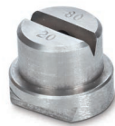
49803 Spray Tip Flow rates from .017 to 7.0 gpm at 40 psi (.064 to 26.5 lpm at 2.8 bar) Self-aligning tip with round top and dovetail connection: spray flow is 5° from offset
