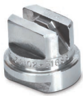
58102 Spray Tip Flow rates below 1 gpm at 40 psi (3.9 lpm at 2.8 bar) Self-aligning tip with wrench flats on top of tip and dovetail connection; spray is offset 5° from dovetail
