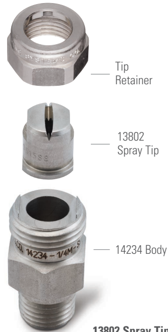
13802 Spray Tip + 14234 Body 1/8" to 1/2" female conn. Flow rates from .009 to 7.0 gpm at 40 psi (.03 to 26.5 lpm at 2.8 bar) Self-aligning tip with wrench flats on top of tip: straight alignment flats connection
