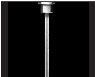
A solid jet of liquid. No atomization occurs. (For illustrative purposes only.)
