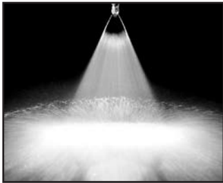
Large free passage design reduces clogging and produces medium-sized drops.
