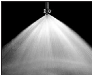
Full cone pattern with relatively coarser drops.
