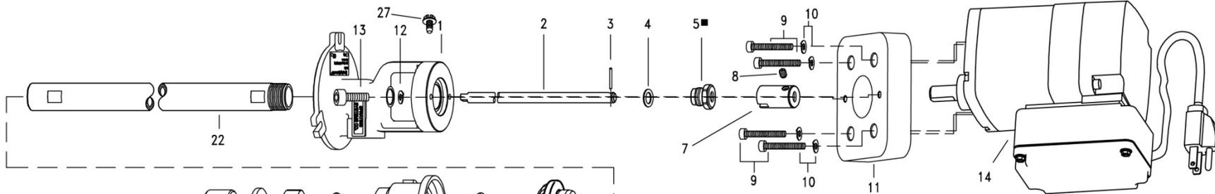
■ NOTE: SEE TORQUE REQUIREMENTS AND LOCTITE NOTES FOR REASSEMBLY OF THE PARTS
