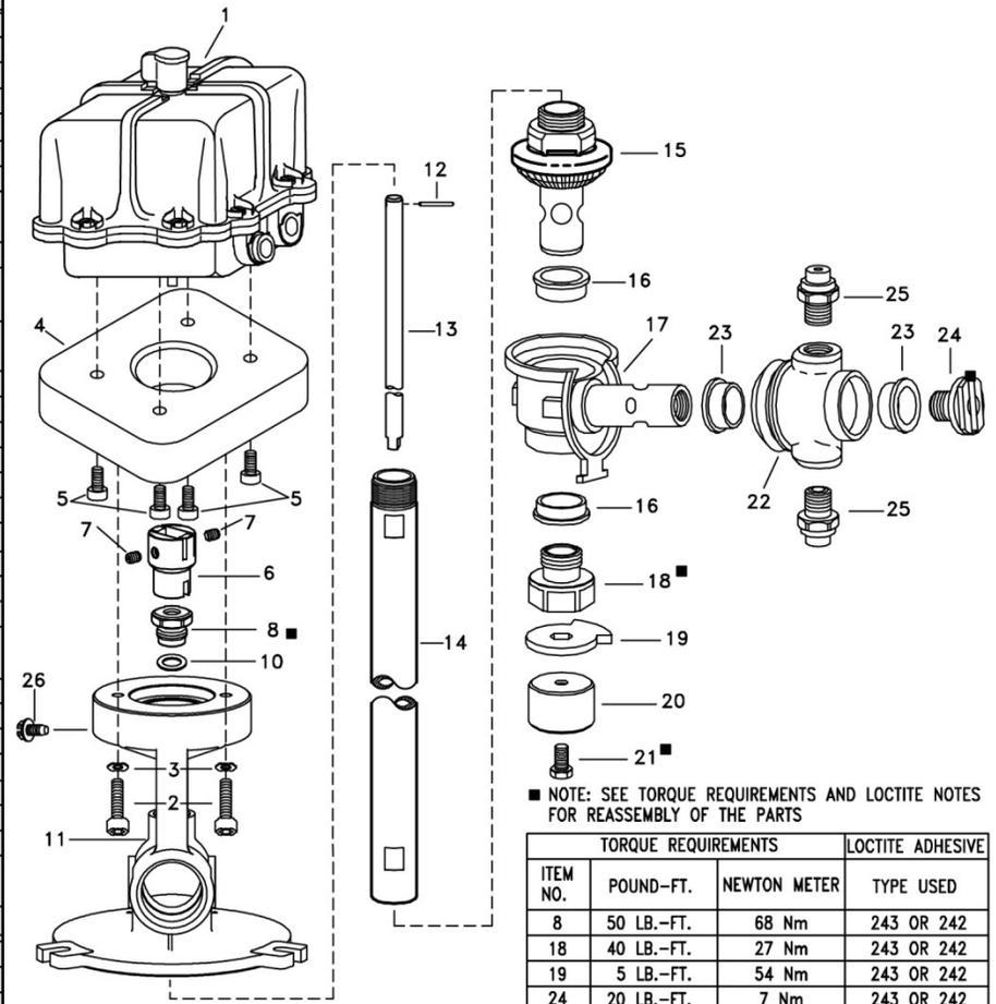
■ NOTE: SEE TORQUE REQUIREMENTS AND LOCTITE NOTES FOR REASSEMBLY OF THE PARTS
