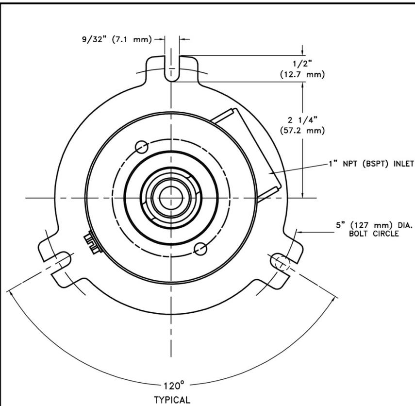
**MOTOR END VIEW OF INLET BODY MOUNTING FLANGE**
