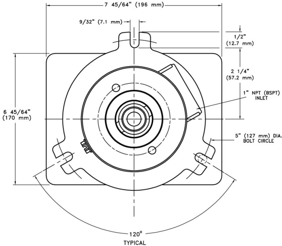
**MOTOR END VIEW OF INLET BODY MOUNTING FLANGE**
