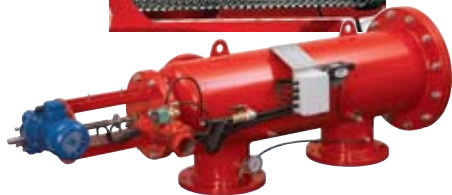
One type of self-cleaning strainer uses a suction scanner, a hollow stainless steel pipe with tubular nozzles evenly spaced along its length. The spiraling motion of the nozzles cleans 100% of the strainer screen.
